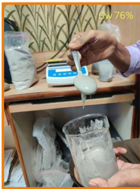
Fig. 5. Paste fill preparation using fly ash
