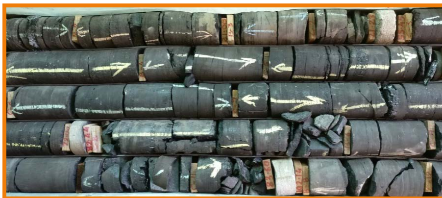
Fig 1. Band by band separation of coal seams
