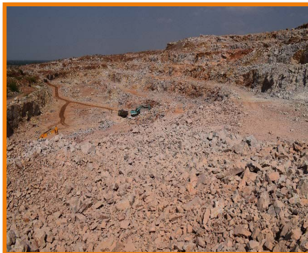
Photo: Blast Induced Ground Vibration Study at Silica Sand Mines & Fragment Size of Blasted Bench, Easily Handled with low capacity Excavator
