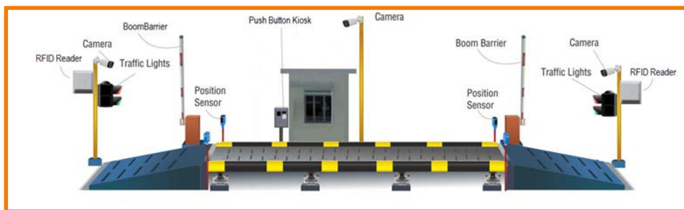
Fig. 2.2.1: Schematic diagram of weighbridge automation system
