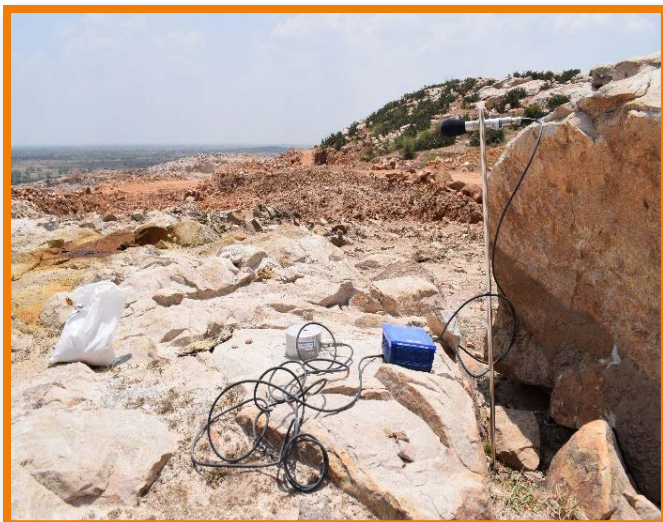
Photo: Blast Induced Ground Vibration Study at Silica Sand Mines & Fragment Size of Blasted Bench, Easily Handled with low capacity Excavator
